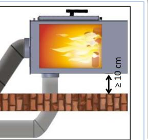
External air intake vents air into the combustion chamber. This is mandatory to use in buildings that are very airtight (buildings with non-closable vents). If external air intake cannot be used then there must be an space of at least 10 cm between the stove and the rear wall so the appliance functions correctly.
